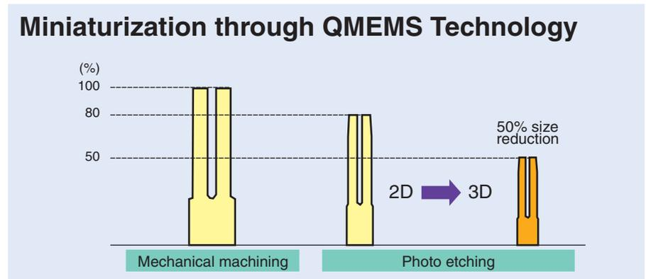
Photo etching technology enables a 20% reduction in the size of tuning fork crystal units. Applying 3D MEMS technology can further downsize the devices to half their former levels without sacrificing stability or precision.
