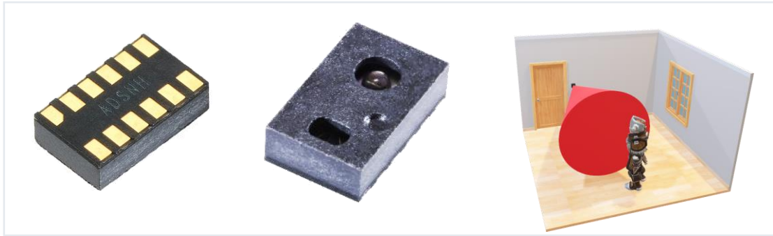
A single zone time of flight sensor
