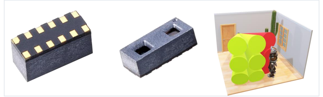
A multiple zone time of flight sensor
