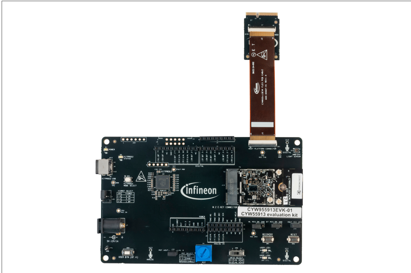
Figure 41 Host interface connection to external host platform
